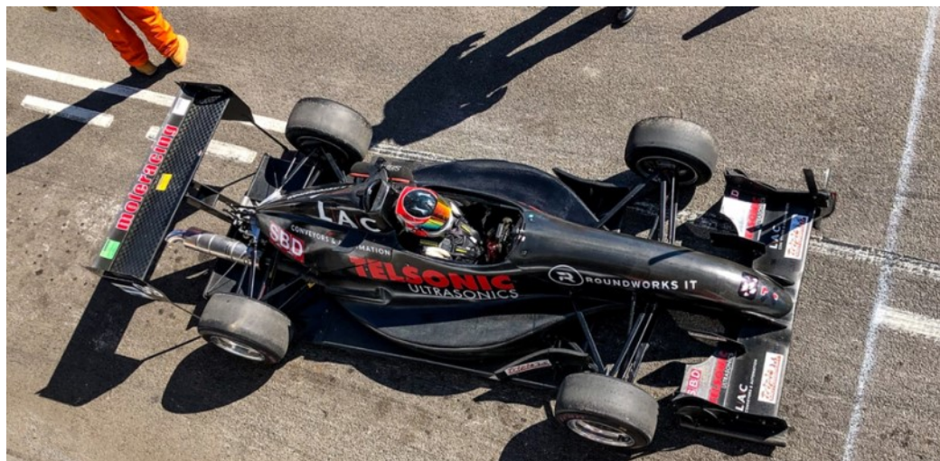
A Formula Ford with homemade downforce additions
