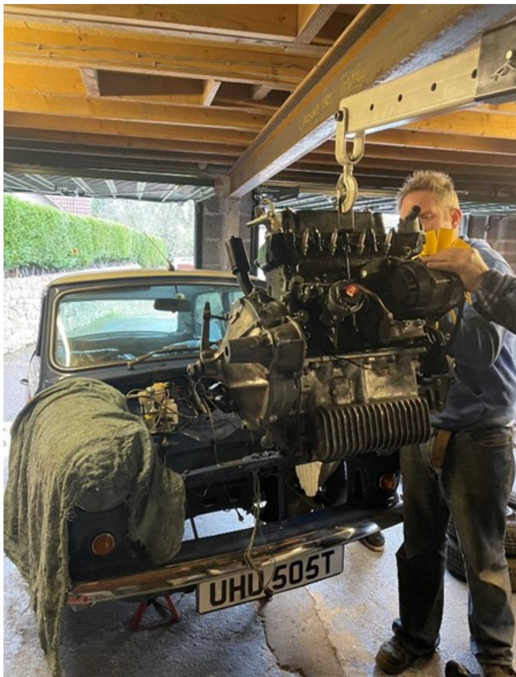
Simon Harris built engine plus box going back in
