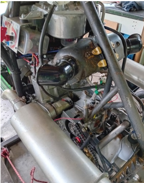
Sealed airbox improved response
