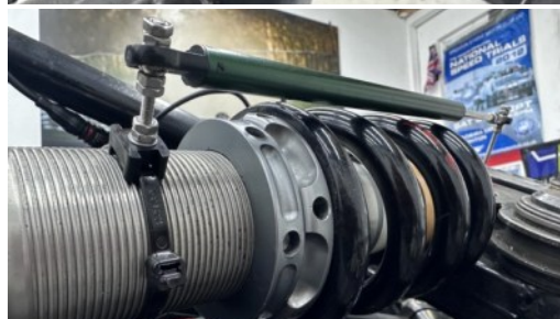
Winter upgrades included new throttle bodies to improve driveability, updated traction control and linear potentiometers on the suspension
