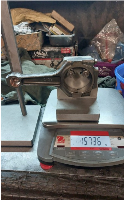
Rods checked for straightness, matched and weighed to +/- 0.1g
