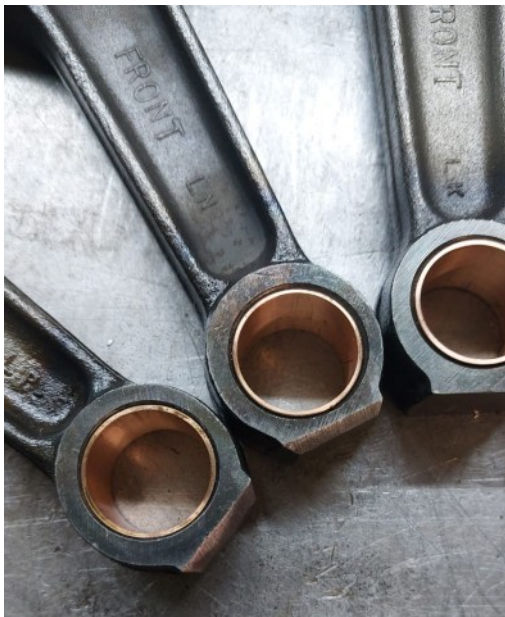
Local specialist machined up phosphor-bronze bushes to cater for -1mm undersized Accralite gudgeon pins
