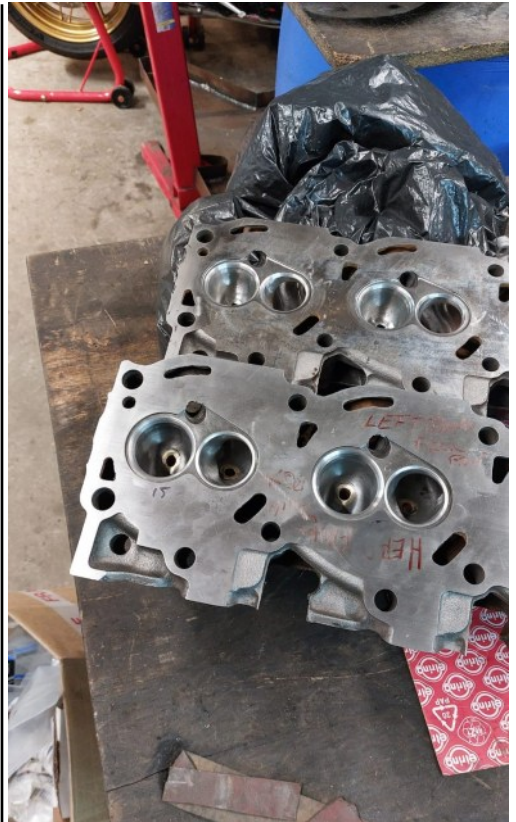
Both heads received new valve seats after discrepancies were found. Opportunity to increase inlet valves to max 46mm
