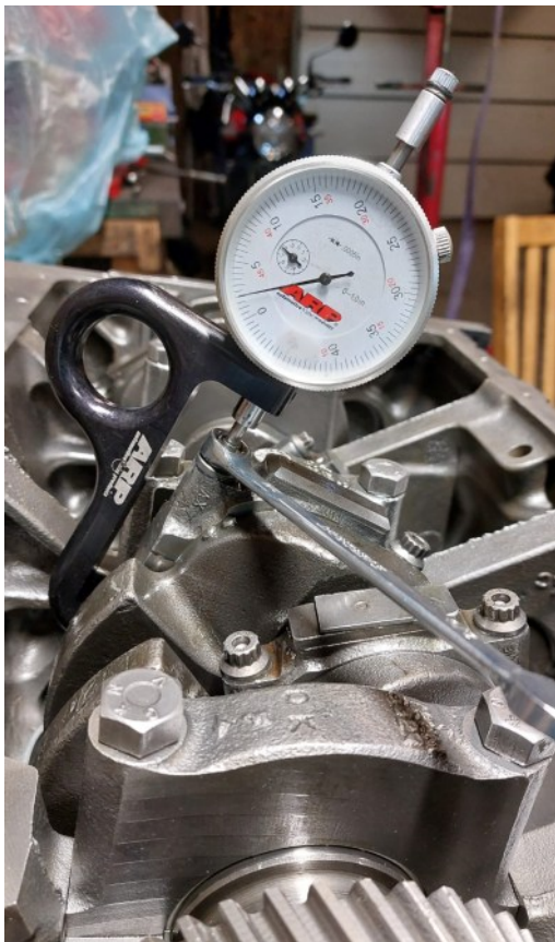
Using a stretch gauge to tighten the ARP big-end bolts
