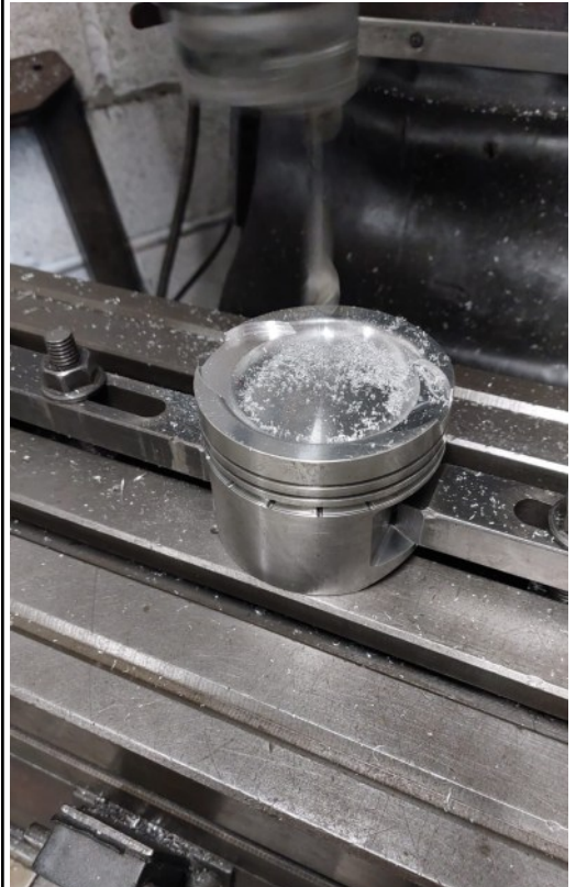
Accralite pistons getting pockets widened for new 46mm inlet valves
